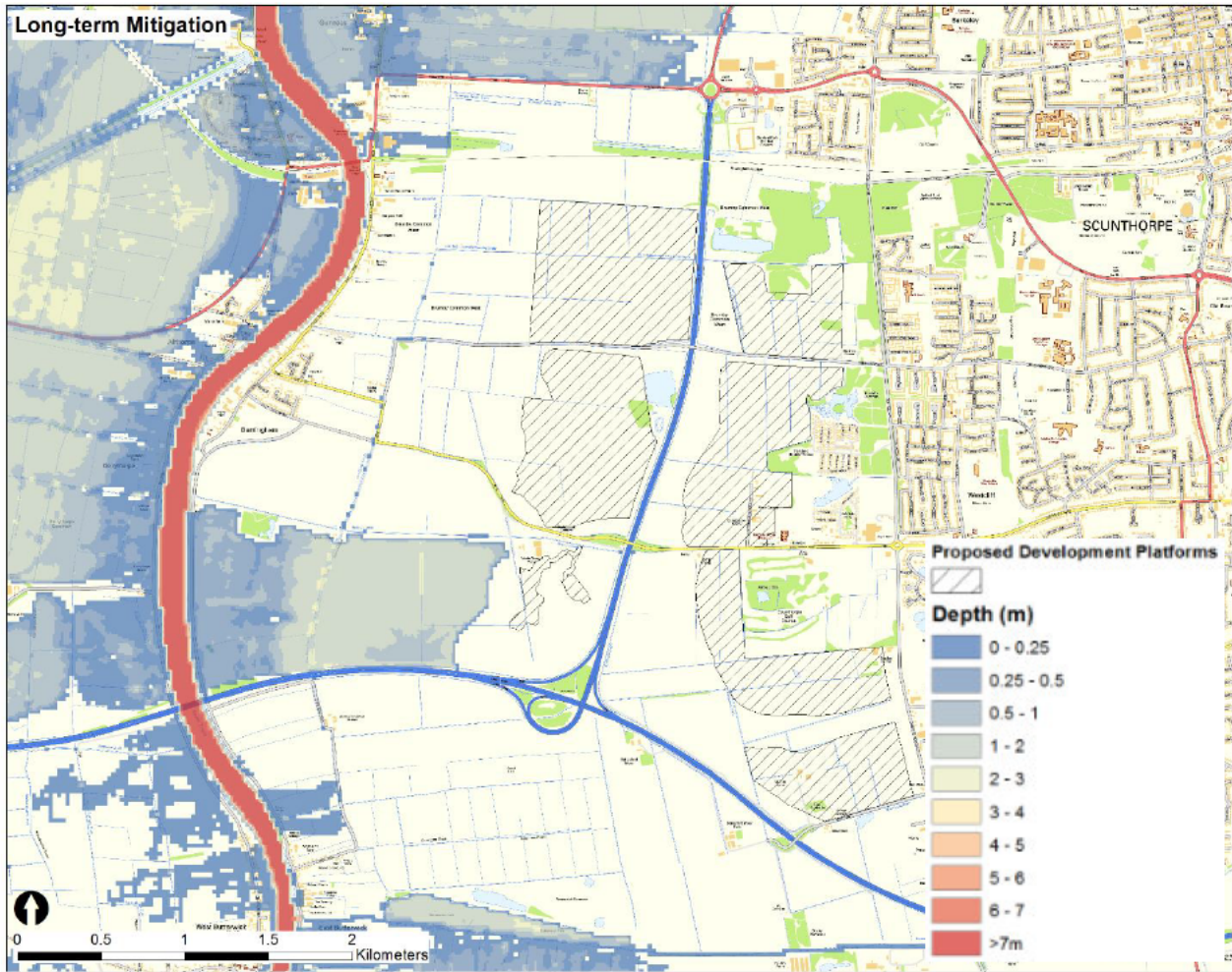
Figure 27: Long-term mitigation works flood depths for 0.5% AEP fluvial event, 2115 with upper end climate change projection
