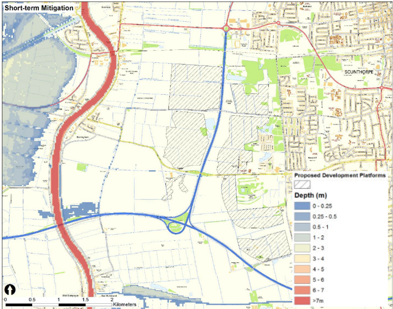
Figure 18: Short-term mitigation works flood depths for 0.5% AEP fluvial event, 2040s with higher-central fluvial and upper end tidal climate change projection
