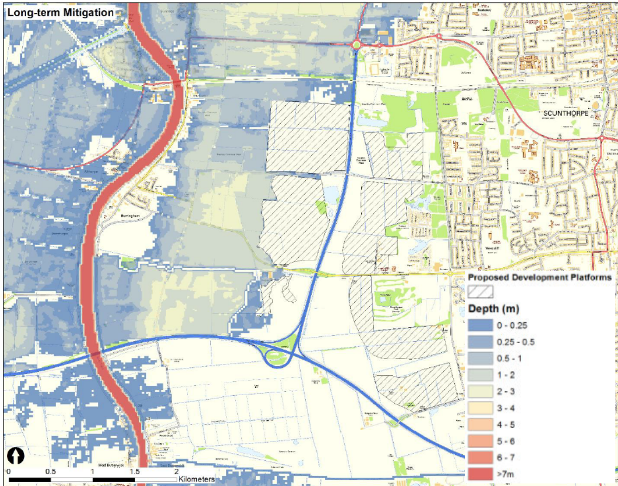
Figure 30: Long-term mitigation works flood depths for 0.5% AEP tidal event, 2115 with upper end climate change projection
