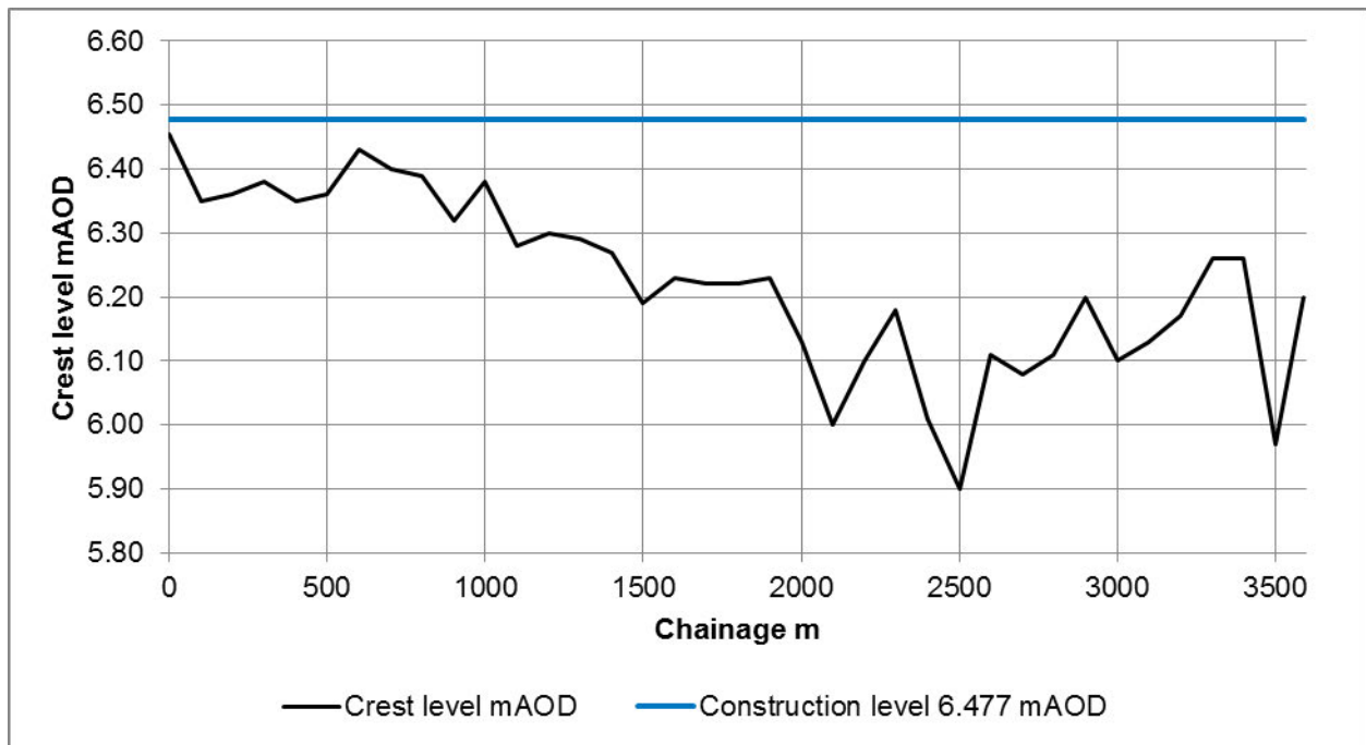
Figure 2: Variation in flood defence height with chainage in relation to the ‘blue book’ level
