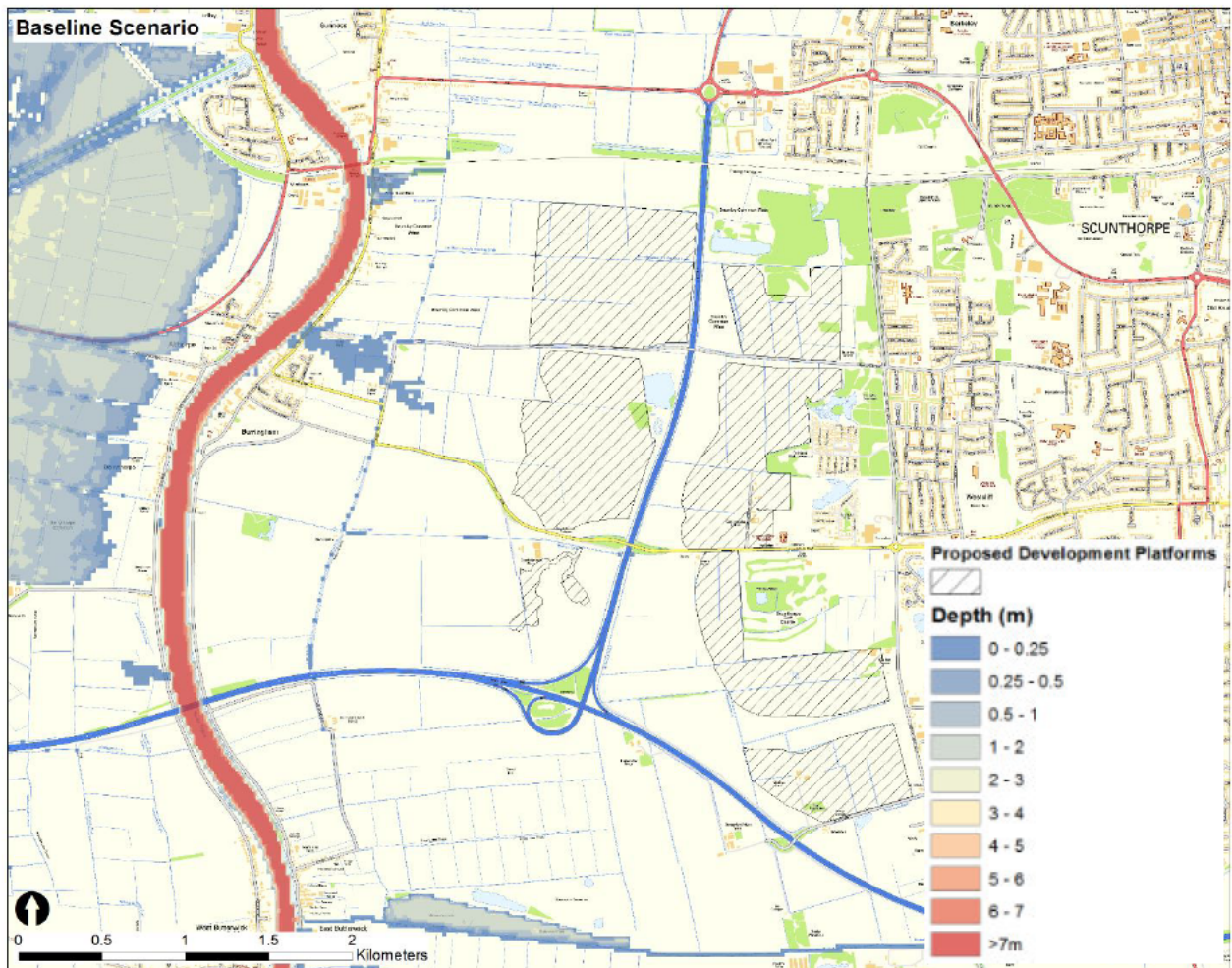
Figure 17: Baseline flood depths for 0.5% AEP fluvial event, 2040s with higher-central fluvial and upper end tidal climate change projection
